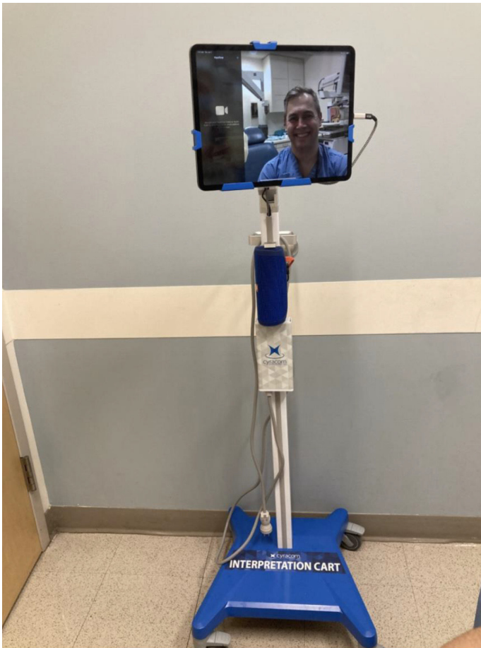
Figure 1. A tablet computer with webcam capabilities mounted on a rolling stand to facilitate virtual outpatient clinics.
